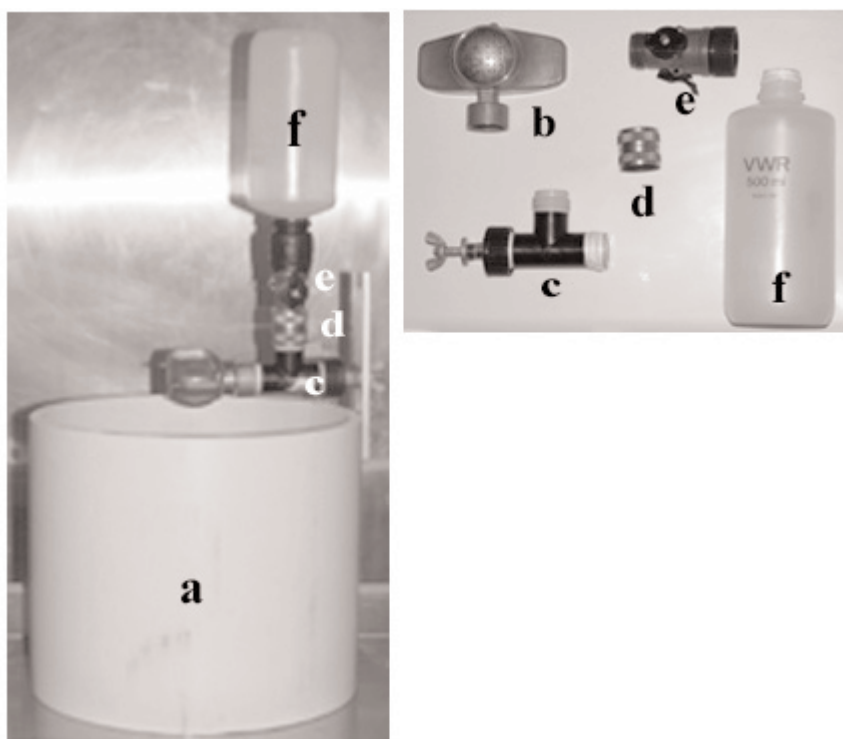
Fig. 1. Treatment applicator developed to apply liquid treatments used a 10-in diameter PVC pipe (a); a garden hose sprinkler (b); three garden hose adaptors (c, d, e), one of which had an on/off switch (e); and a 500 ml bottle (f). The sprinkler system was set at a height of approximately 10 in.
