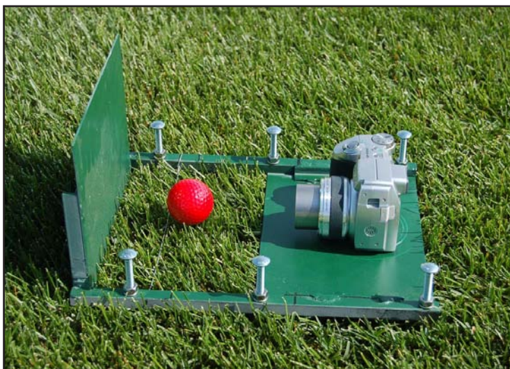
Fig. 1. Device used to collect images of a golf ball resting in the turf and later analyzed using digital image analysis.
