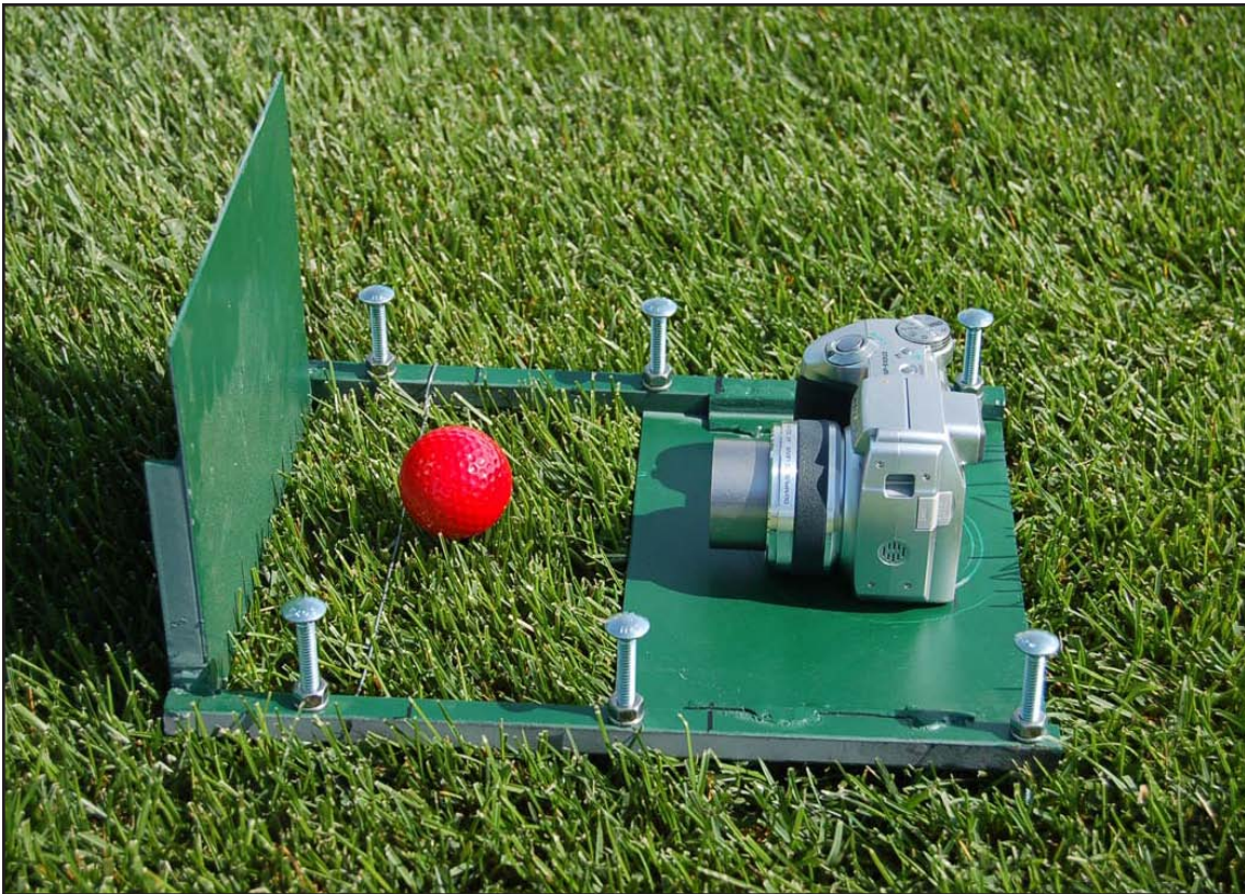
Fig. 1. Device developed at the University of Arkansas to collect digital photos of golf ball lie, which are subsequently analyzed using image analysis software.
