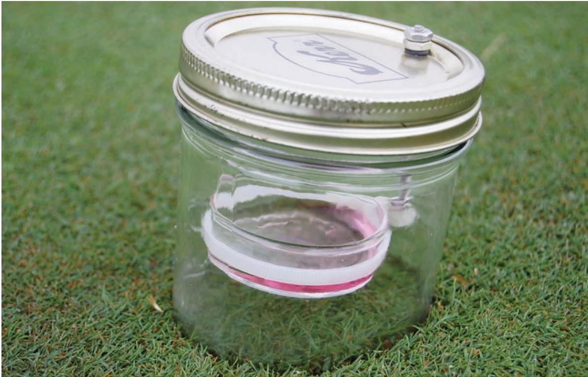
Fig. 1. Apparatus used for in-field ammonia volatilization estimates.
