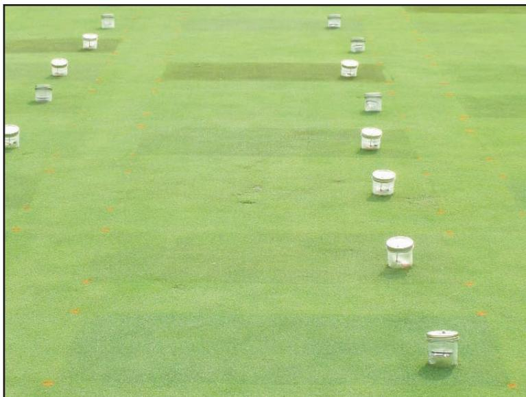
NH<sub>3</sub> volatilization traps installed on plots
