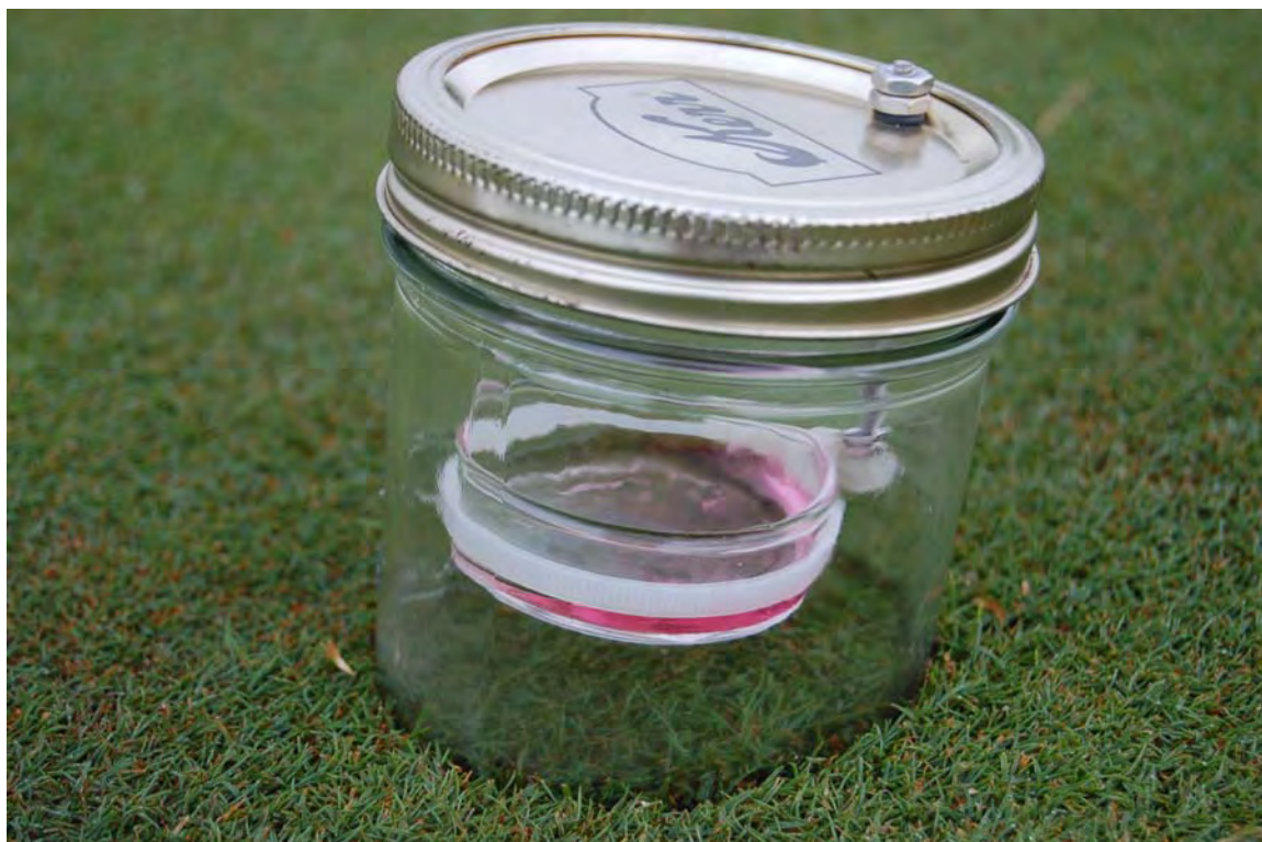
Fig. 1. Apparatus used for in-field ammonia volatilization estimates.
