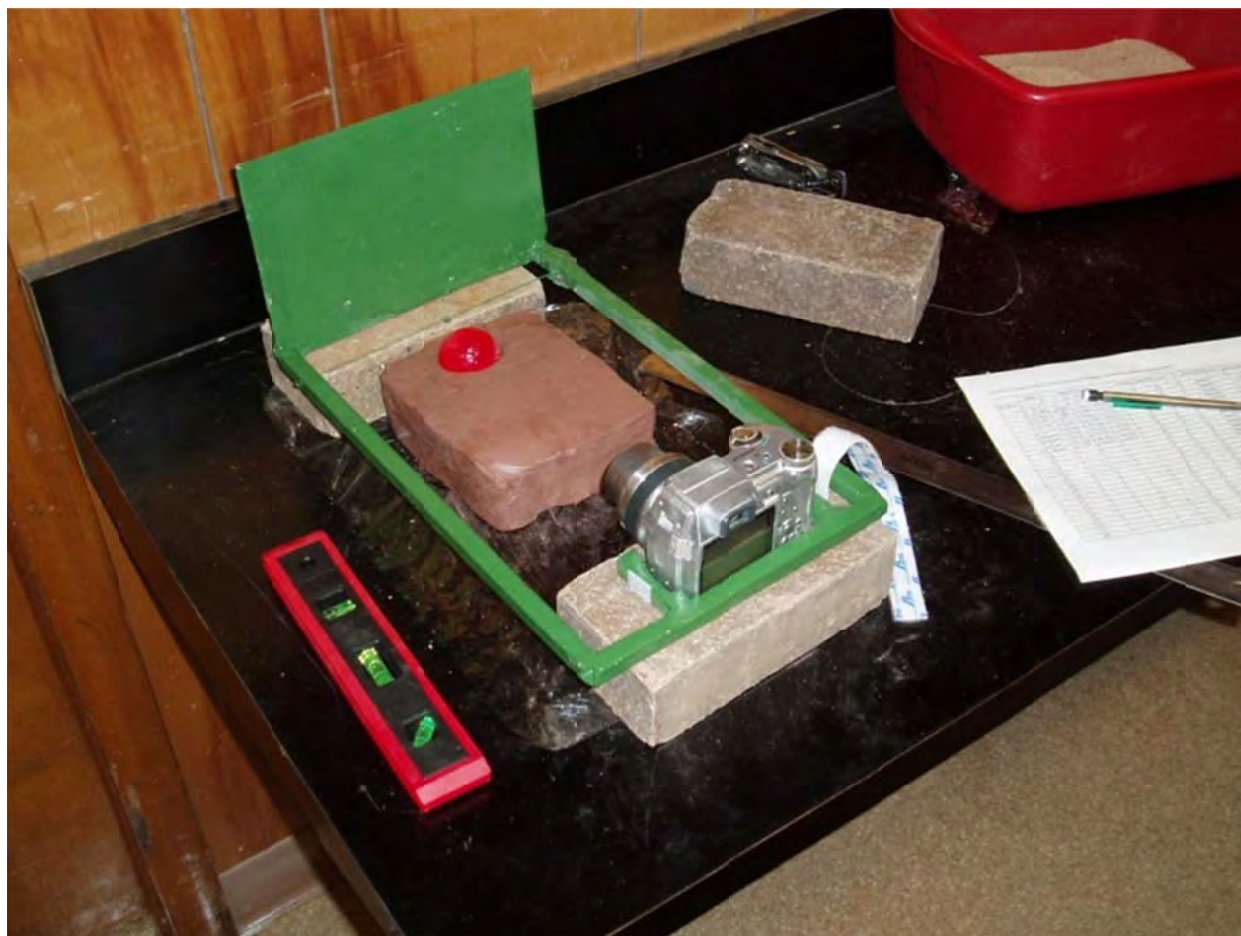
Fig. 1. Setup used for preliminary study to determine if the newly designed frame could successfully measure ball mark severity.
