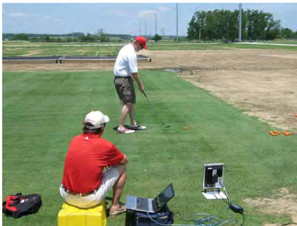
Fig. 1. Coach Adams of the lady Razorbacks golf team operating the Flightscope Kudu as the 0 handicap golfer prepares to strike the golf ball. Ball lie has already been measured.
