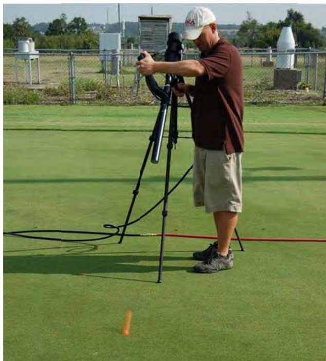
Fig. 2. Pneumatic golf ball launcher designed to fire golf balls from a consistent height and angle required to differentiate ball mark severity in plots subjected to various management practices.
