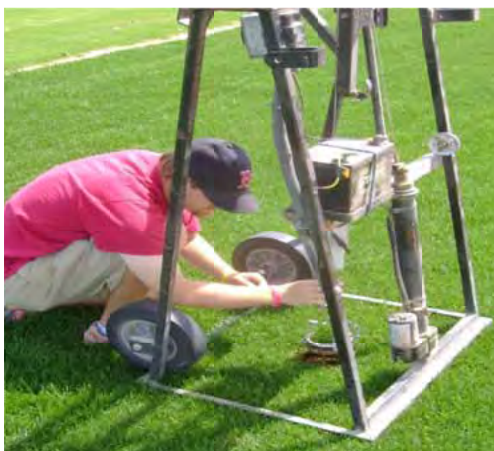
Fig. 1. Sod ring pulling device used to measure root strength by vertical detachment.
