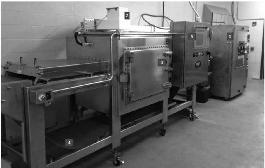
Fig. 1. Industrial-type microwave system used in the study showing the transmitter (1), wave guide (2), heating zone (3), conveyor belt (4), and control panel (5).
