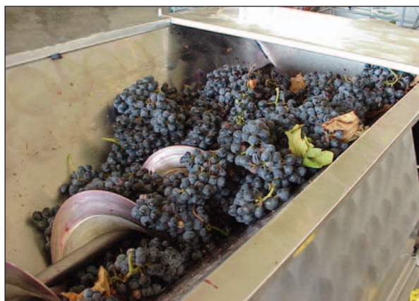
Figure 3. Destemming/crushing equipment removes the grapes from their stems and crushes the fruit to release the juice.
