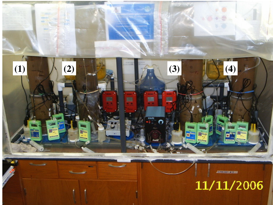
(a) Column experimental setup. (1): Continuous flow column, (2): Pre-treatment column, (3): Oxidic water-level fluctuation column, (4) Anoxic water-level fluctuation column
