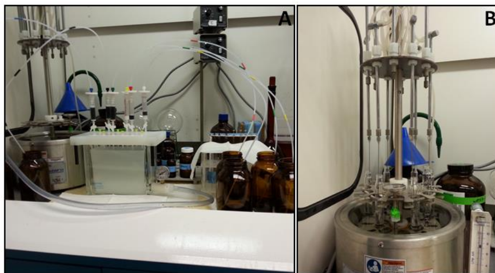
Figure 2: (A) Solid phase extraction setup; (B) Sample concentration apparatus.
