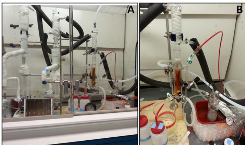
Figure 1: (A) TONO assay setup with liquid-liquid extraction apparatus; (B) TONO assay setup.
