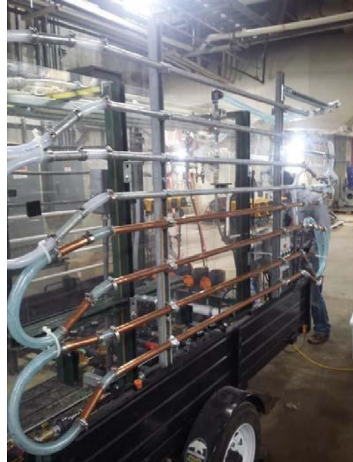
Figure 3: Pipe loop displaying Lead train (top of pipe wall) and PVC train (bottom of pipe wall).
