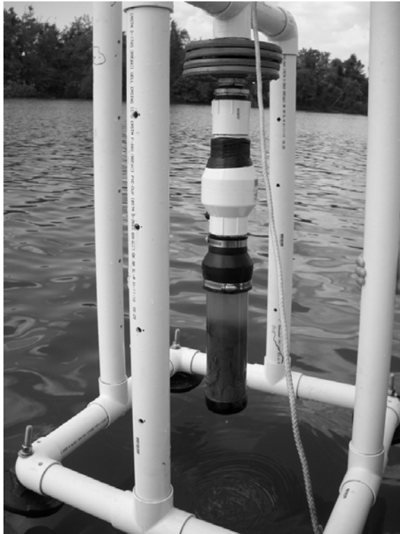
Figure 2. Modified HYPOX (see Gardner et al., 2009) sampler used to collect sediment cores from Lake Wister for sediment O 2 demand and P release rates, as measured in the laboratory.
