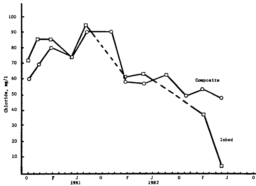
Figure 49. Chloride in the composite and the inbed wells of the 02MG30 filter field.
