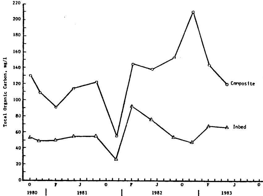
Figure 11: TOC of the composite and inbed wells of the 01ST76 filter field.
