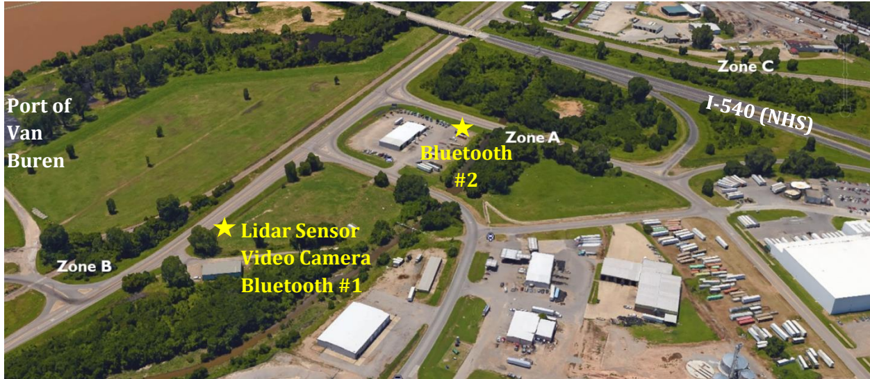
Figure 8 Overview of Van Buren sensor set-up
